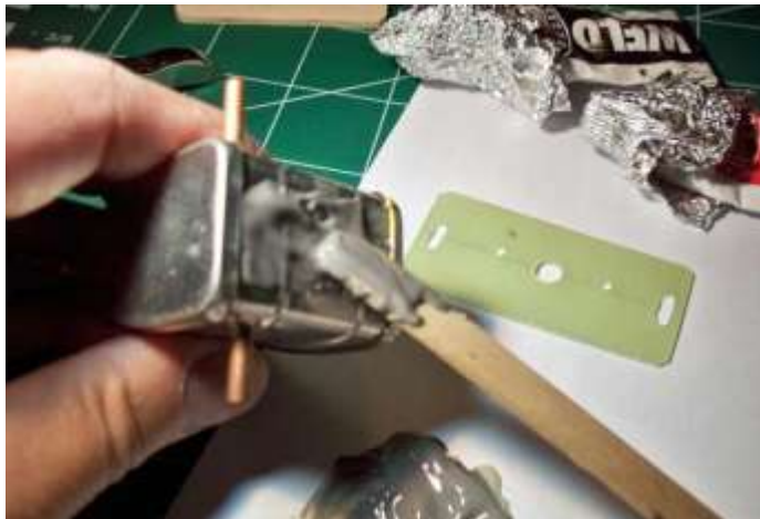
Glue the tank to the mount using J. B. Weld epoxy glue.
