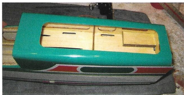
Front wheel well depth is restricted by the tank bay above so it cannot not be increased
