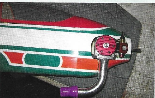
Cutting out a neat hole for the engine and carburettor using a paper template and transferring the shape developed to the glassfibre cowl
