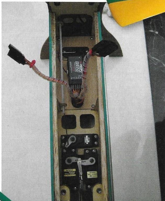
Radio fit using some pre-digital but good quality coreless JR servos
