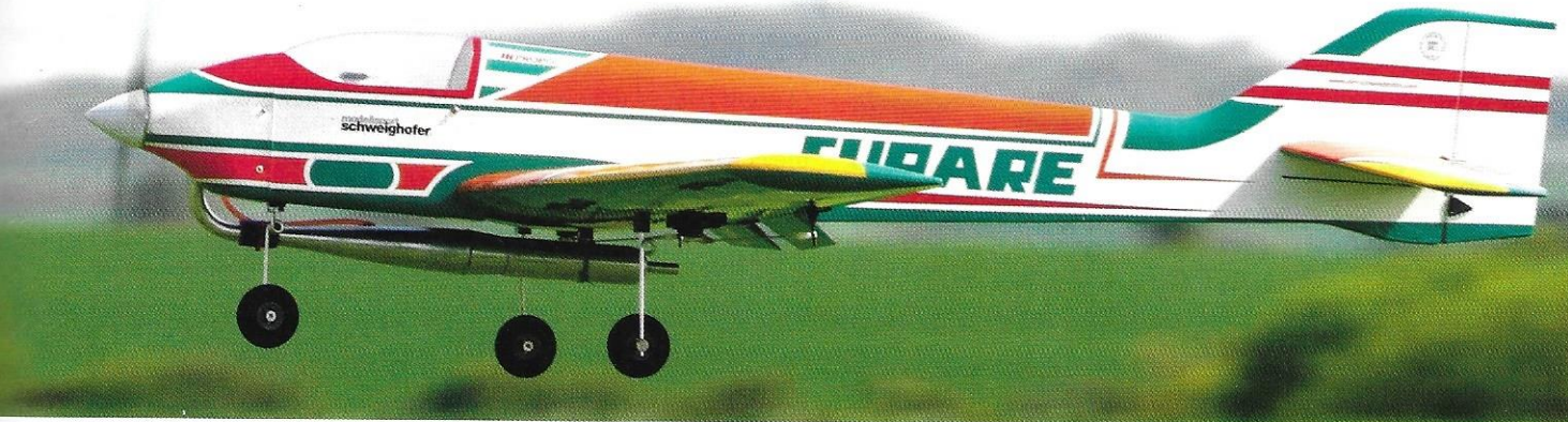
Landing flap allows you to come in with a bit more power and touch down at your feet at low speed every time
