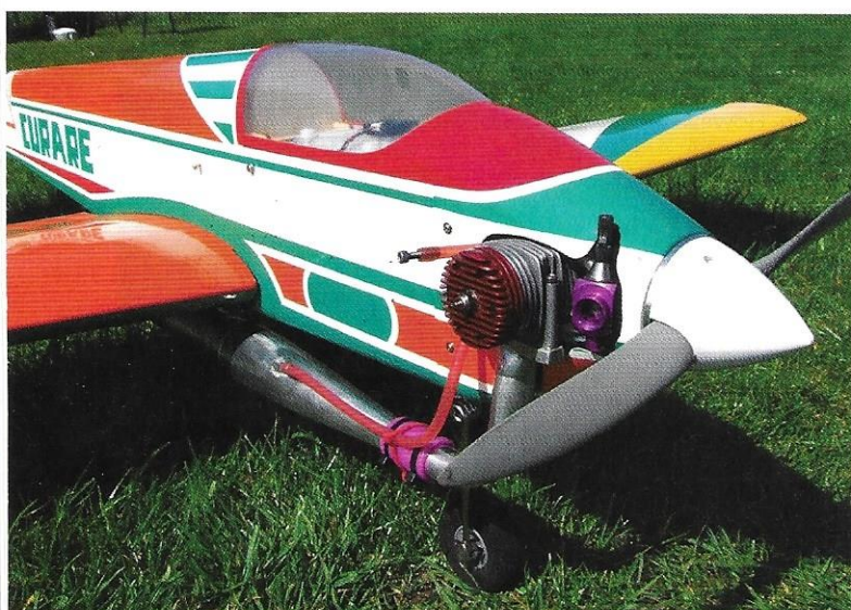
The West 52 and matching pipe, manifold and large propeller give very reasonable noise levels with linear throttle response and lots of power!
