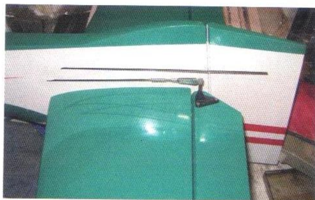
Connecting up the tail linkages using good quality parts
