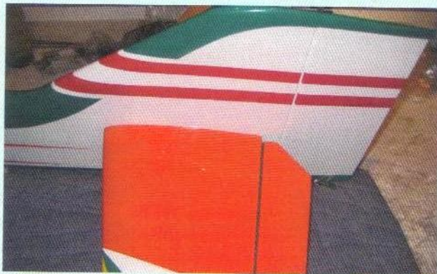
The anhedral tail is joined using a short ply brace and a carbon rod incidence peg fitted into pre-formed slots in the fuselage
