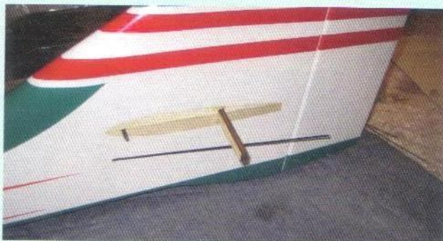
The anhedral tail is joined using a short ply brace and a carbon rod incidence peg fitted into pre-formed slots in the fuselage
