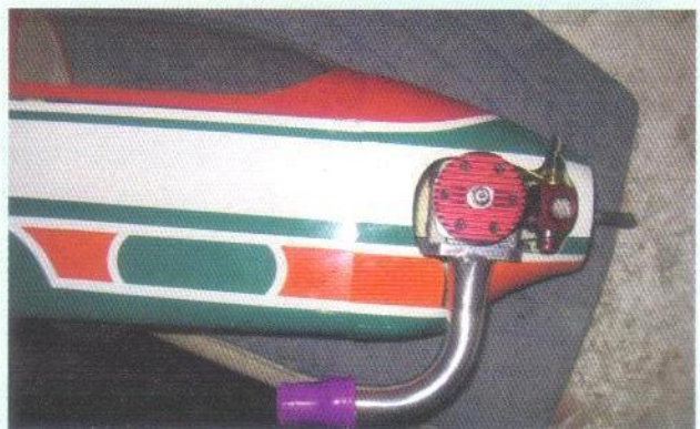
Cutting out a neat hole for the engine and carburettor using a paper template and transferring the shape developed to the glassfibre cowl
