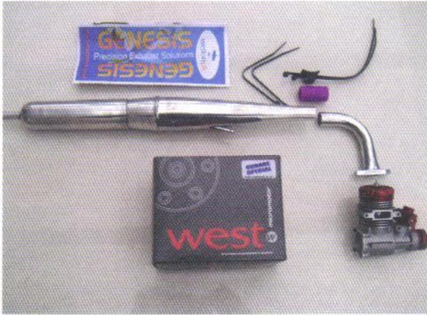
Optional West Eurotech 52 T1 'Curare Special' engine with matching Genesis tuned pipe and manifold
