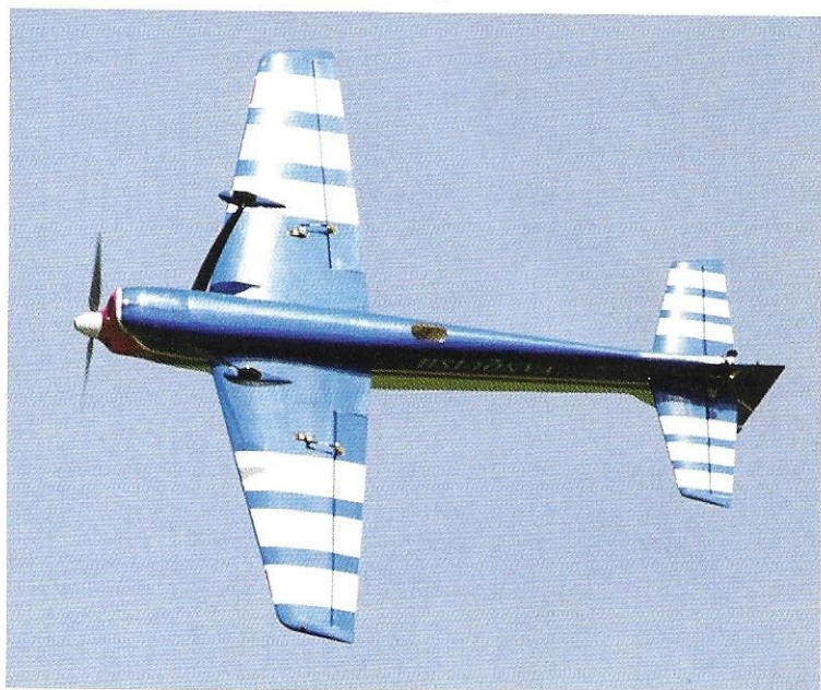
BELOW At maximum stick deflection I set-up the maximum response I need. On ailerons this is during a roll at the top of a manoeuvre when the airspeed is at its lowest. Then use exponential to reduce sensitivity around centre
