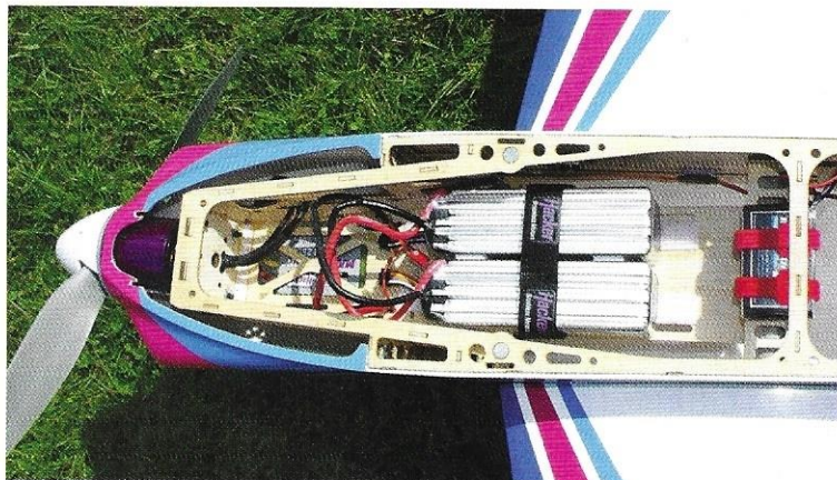
ABOVE: Jon's installation uses twin 5-cell Thunder Power packs connected in series. There's plenty of room to move the LiPo's to experiment with different C of G positions
