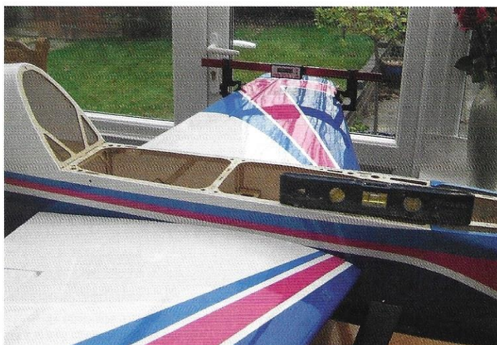
On the Vanquish the zero datum line is the top deck of the fuselage, continually checked using a spirit level while making incidence adjustments
