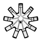
A radial engine uses a master with slave Con-rods, When you study the theory and geometry differences on each connecting rod you discover there are small differences in stroke and hence cubic capacity on each cylinder. This explains why at idle, a radial engine has that characteristic fluctuating exhaust note.
