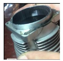
Saito production engines tend to run weak and hotter on the upper (no1) cylinder then richer and cooler on no 2 & 3. There are many reports of cylinder bases cracking on no 2 & 3. considered to be caused by excess fuel ingestion and hydraulic locking in certain conditions.
