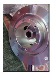
The factory fuel mixture distribution plenum can suffer from neat fuel "pooling" which can be ingested into one of the lower cylinders causing hydraulic lock. The following pic shows the radially drilled passages to the cylinders .
